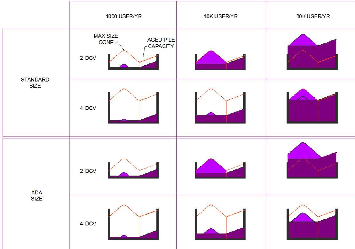
Figure 1. Graphical representation of the TTS Decompose DCV fullness after 10 years of light, moderate, and heavy use (light purple shows portion of maximum sized fresh waste cone filled in a year, dark purple shows portion of DCV filled after 10 years).
